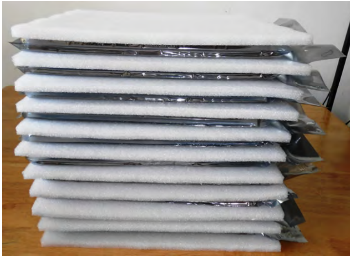
Place Foam Sheets Between Trays
